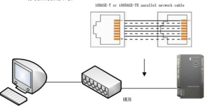
(2) Communication line connection between BACnet gateway and AC units: When gateway is connected to main control unit of ODU, ODU with the address dial-up of 0 must be connected.
