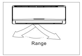
Adjust the air flow direction properly, otherwise it might cause discomfort or cause uneven room temperatures. Adjust the horizontal louver using the remote controller. Adjust the vertical louver manually or using the remote controller(depending on models).
