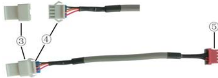
Fig. 24: Schematic diagram of patch cord: Terminal ③ is the protection terminal; connect terminal ④ to the terminal ② of connection wire ; connect terminal ⑤ to the terminal of wired controller of air conditioner
