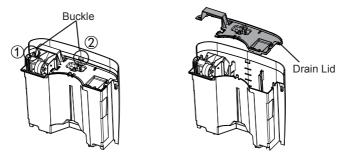
3. After cleaning, replace the drain lid and make sure the float of water bucket is placed properly. The side with foam plastic should be beneath the drain lid. Do not remove the foam plastic on the float.
