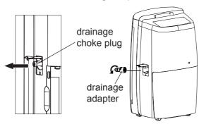
3. Insert the drain hose into drainage adapter to make sure the water won't leak out. The horizontal height of drain hose should not be higher than the drain outlet. Do not block the drain outlet to make the condensate water can be drained out smoothly. Please check drainage adapter and drain hose periodically to see whether they are connected tightly and whether they are damaged or blocked.
